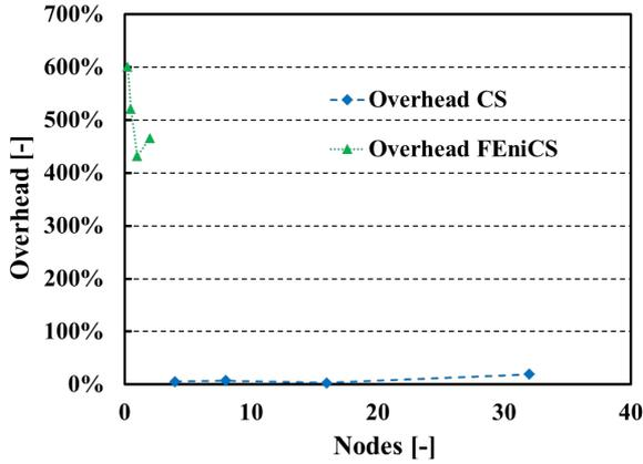
Figure 6 Parallel speedup (a), parallel efficiency (b), the total run time for 100 time steps (c) and overhead for each solver (d) on ParaSiF\_CF with a linear structural solver for 233M cells for the CFD domain and 2.7M DoFs for the CSM domain.
