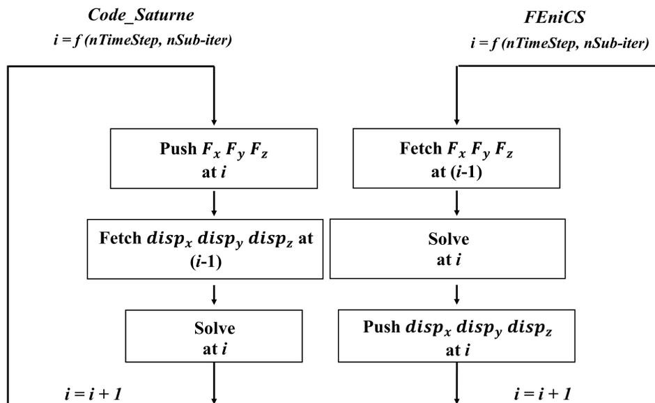
Figure 1 Data exchange scheme through MUI library for Code\_Saturne (left) and FEniCS (right)
