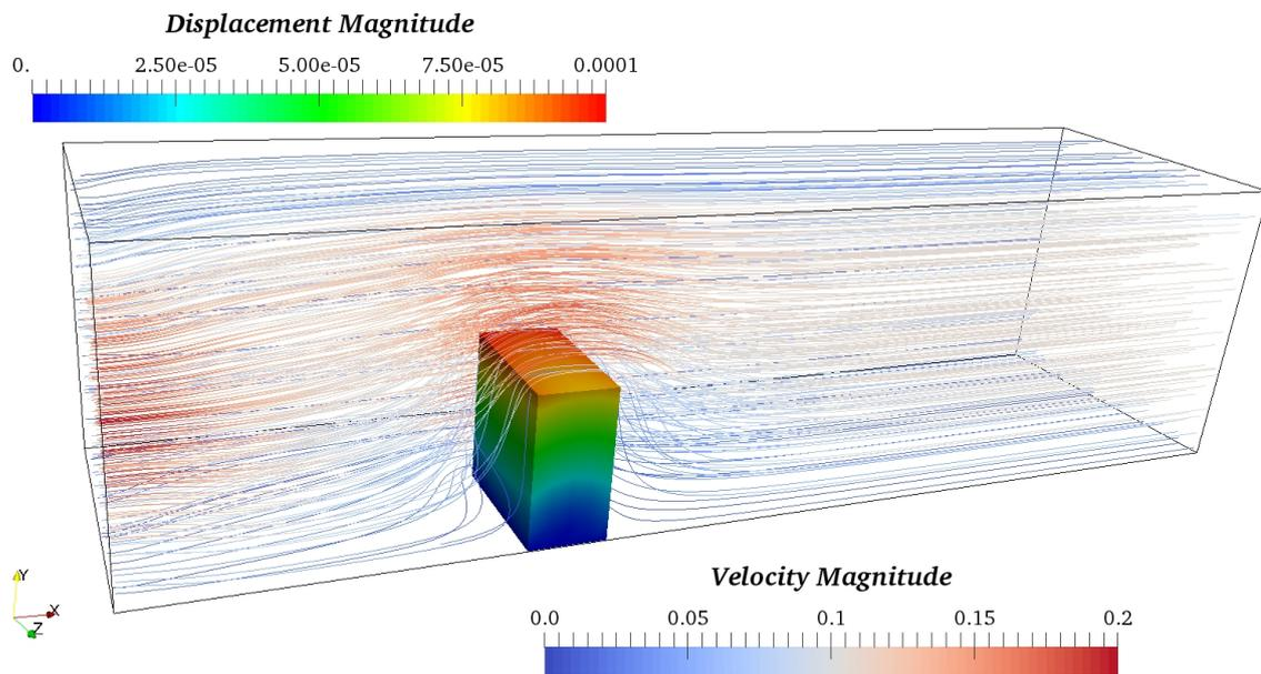
Figure 4 Streamlines (for the fluid domain) and displacement magnitude contour (for the structure domain) for the 3-D flow past an elastic beam using the linear structural solver.
