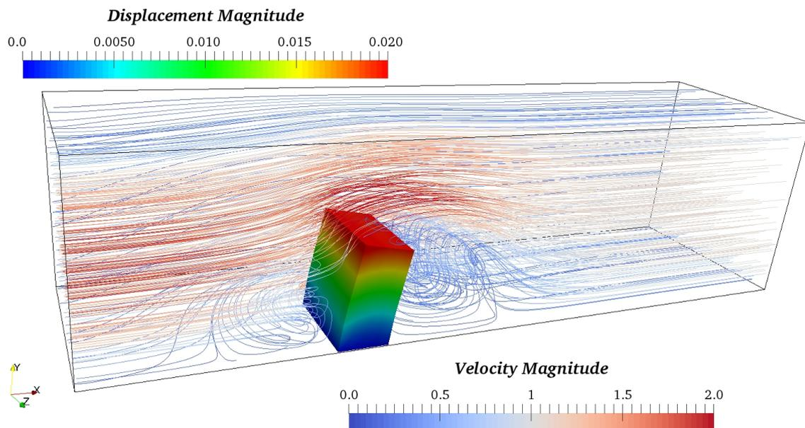
Figure 8 Streamlines (for the fluid domain) and displacement magnitude contour (for the structure domain) for the 3-D flow past elastic beam case with non-linear structure solver.
