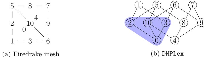
Figure 1: (a) An example Firedrake mesh; global point numbers associated with the cells, faces, and vertices are shown. (b) `DMPlex` representation of the mesh topology; an example adjacency relation is highlighted, where the cell with global point number 0 is connected to the faces with global point numbers 2, 10, and 3.
