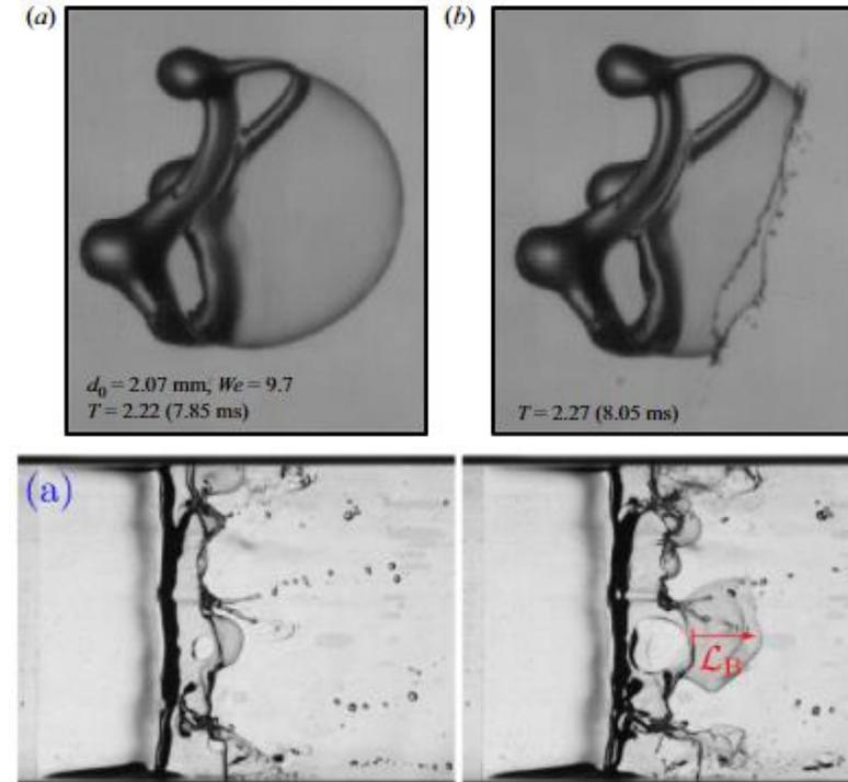
A droplet (upper row) [2] and a wind-sheared liquid film [3] undergoing bag breakup.
