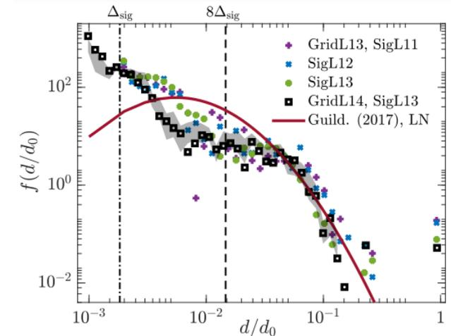
Grid convergence study showing the time- and ensemble-averaged size distribution of aerobreakup fragments without (left) and with (right) the MD algorithm applied. For all cases  $We = 15, Oh = 0.001$ .
