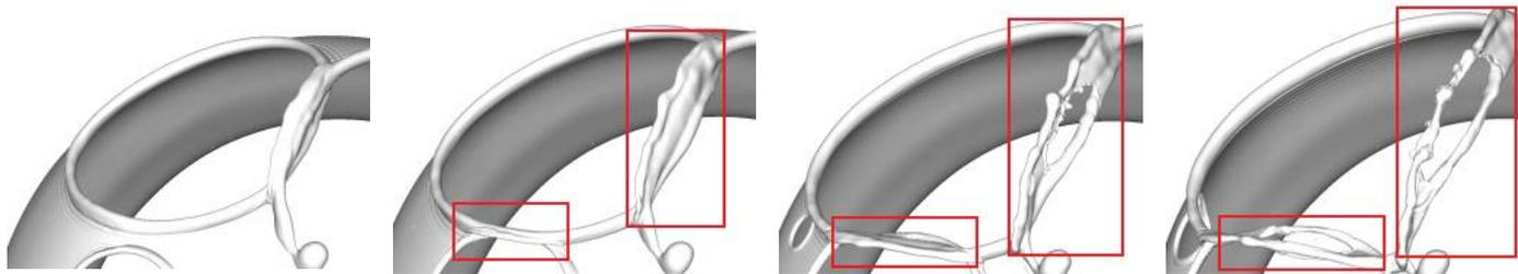
Evolution of 'fingering' liquid lamellae during bag film fragmentation with  $We = 15$ ,  $Oh = 0.001$ ,
