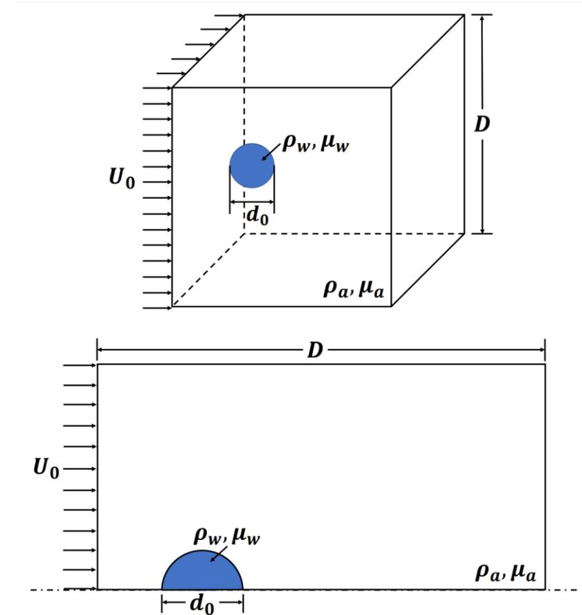
Fig. 5 Sketches showing initial configuration of flow fields in 3D (upper) and axisymmetrical (lower) simulations.
