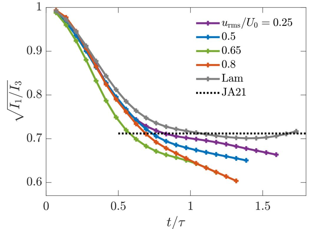
Evolution of mode-2 deformation  $a_2$  (left) and droplet aspect ratio  $\sqrt{I_1/I_3}$  (right)
