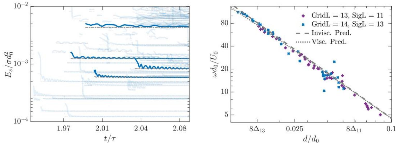
Left: evolution of fragment surface energy; right: frequency of the dominant mode of fragment oscillation as a function of fragment radius, with theoretical prediction of [2] superimposed
