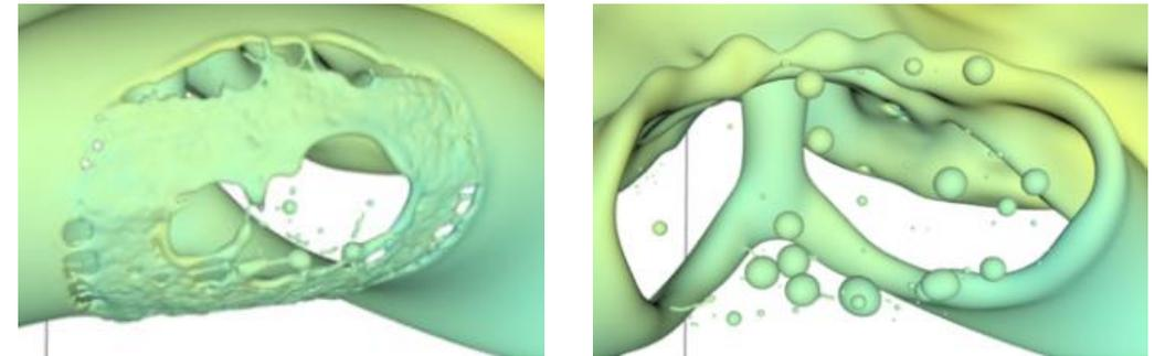
3D atomization simulations with default (uncontrolled) perforation and controlled perforation by the MD algorithm. Upper row: snapshots of present aerobreakup simulations at GridL = 12 and 13; Lower row: snapshots of the phase inversion test from [1].
