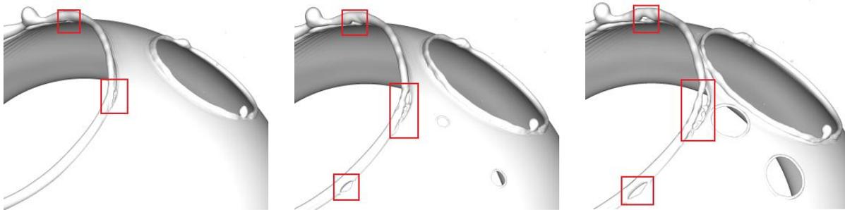
Destabilization of a receding rim on the bag surface with  $We = 15$ ,  $Oh = 0.001$ ,
