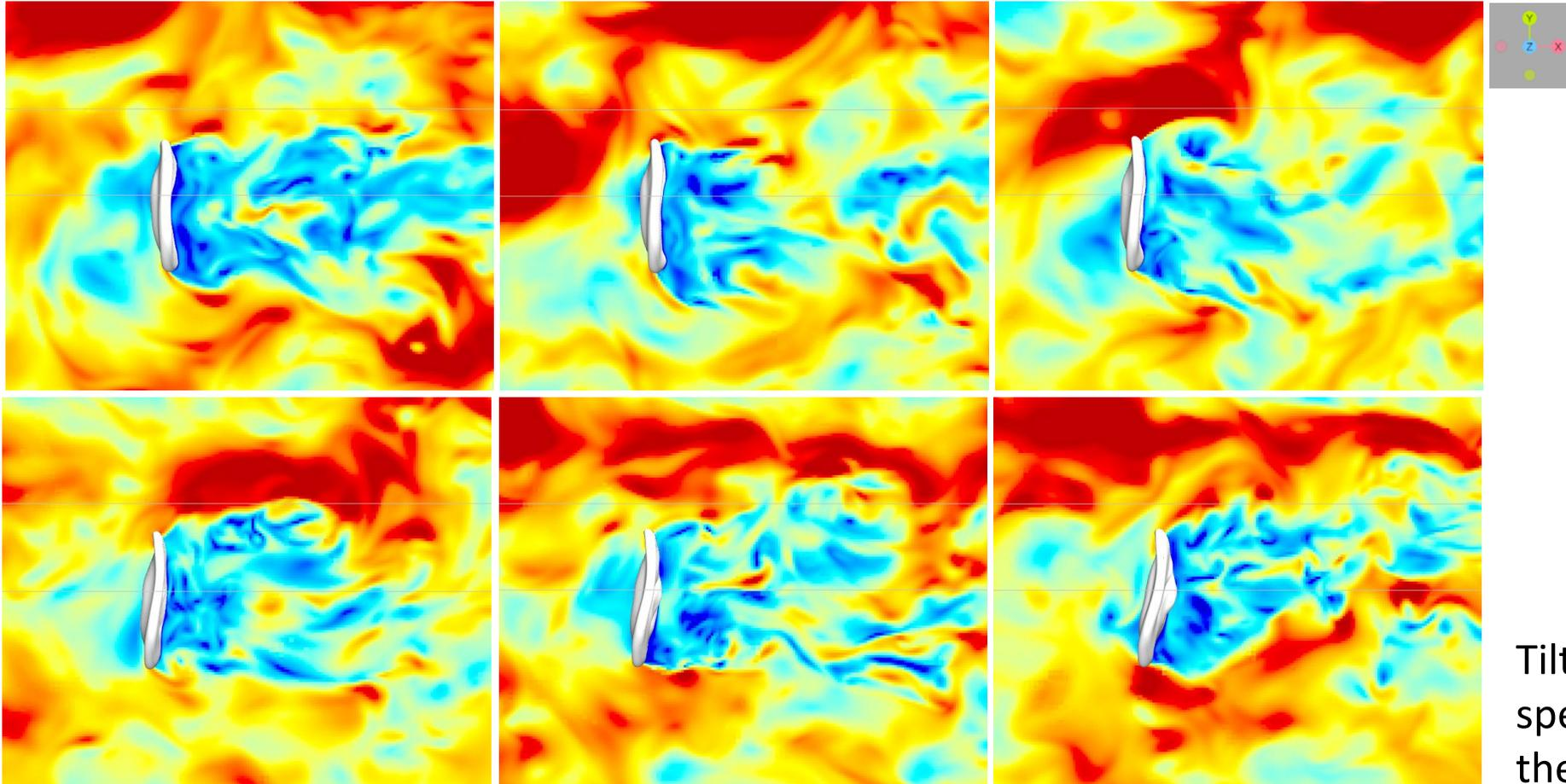
Tilting triggered by high-speed air parcels bypassing the flattened droplet
