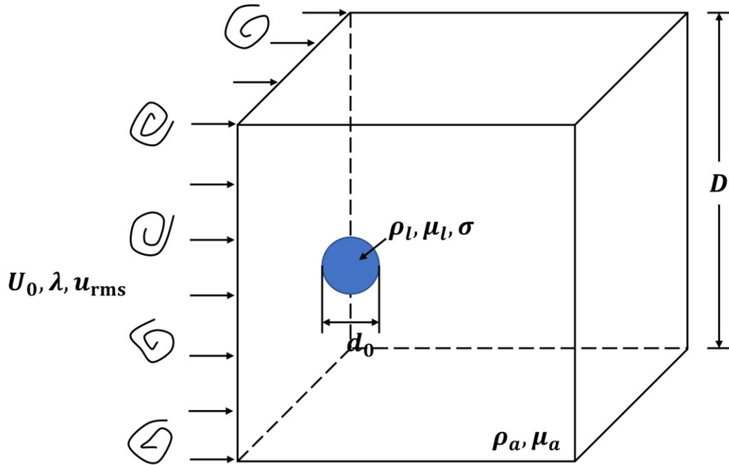
Schematic illustration showing the configuration for the turbulent aerobreakup problem.
