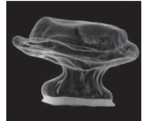
Morphology of breaking droplet and associated fragment size distributions in laminar and turbulent airflows [1][3]
