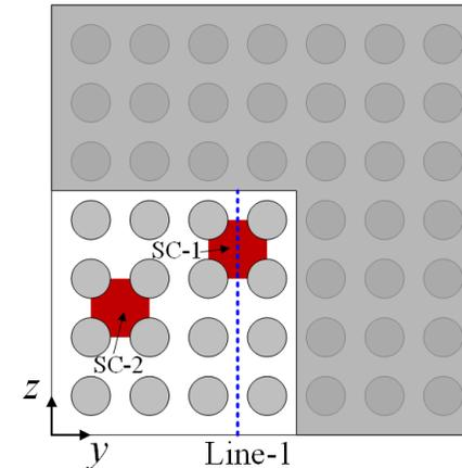
Mean and RMS velocities were measured along horizontal lines (Line-1) of various axial locations [1]
