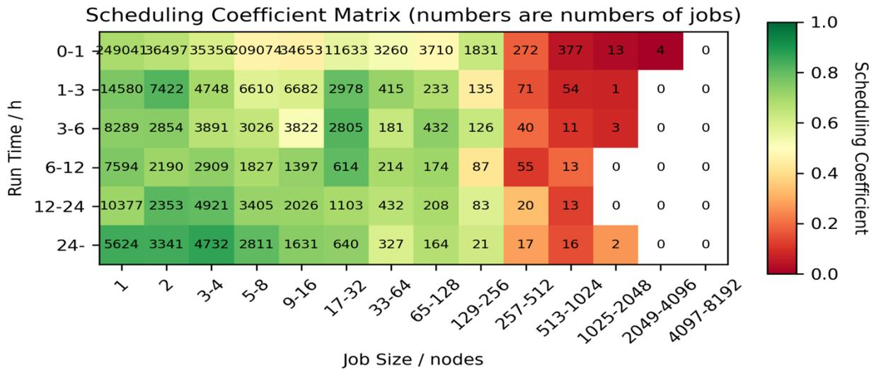
The usage heatmap below provides an overview of the usage on ARCHER2 over the quarter for different job sizes/lengths. The colour in the heatmap indicates the number of CUs expended for each class, and the number in the box is the number of jobs of that class.
